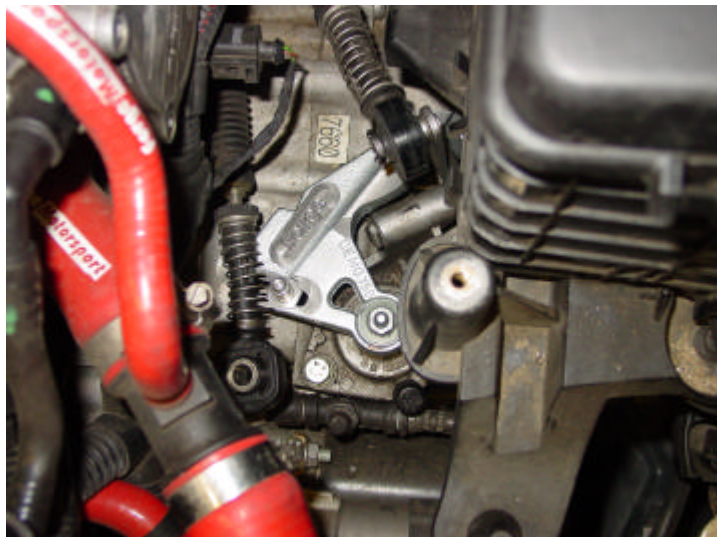
New short shift partly fitted to vehicle.
