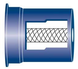
greaseable shackles as the grease can travel from the centre of the bush along the helix and out to the grease grooves in the head of the bush.
