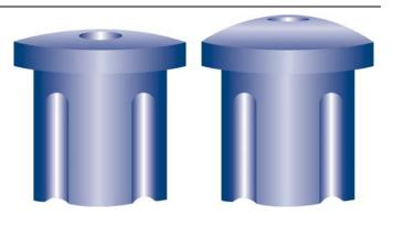
polyurethane is in a solid form when it is manufactured into bushes, its unique properties enable it flow in a manner similar to a liquid when loaded. The action of the bush flowing into its voids prevents the generation of harshness and NVH within the bush and its mount.
