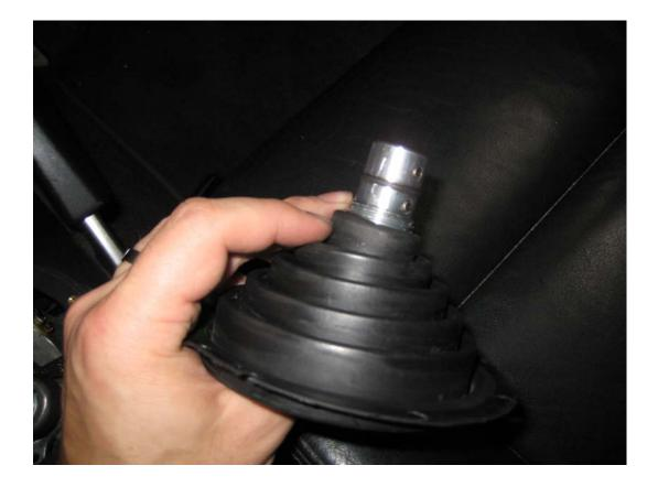
4. Replace over the shifter rod and push down until the distance between the top of the shifter rod and the top of the Forge adaptor is approx. 28mm (NB: depending on how many threads you managed to push though the gaitor, this dimension may be slightly lower or higher, however this is a good starting point)
