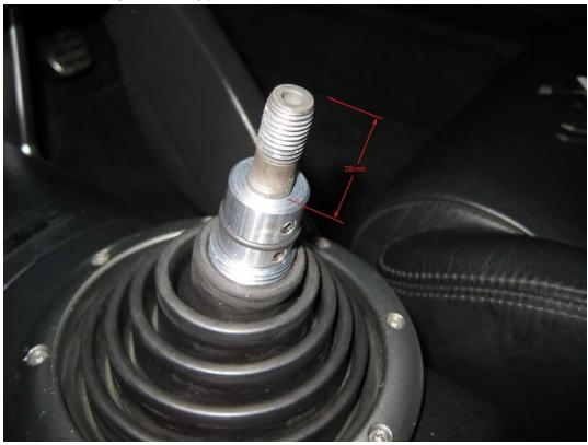
....then tighten the grub screws to hold the adaptor to the gear stick.
