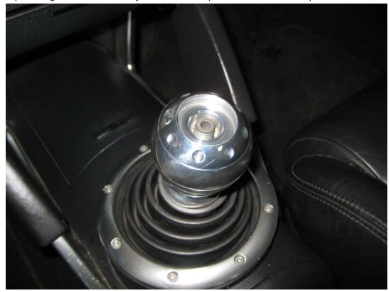
6. Add the shift pattern top cover to the knob, ensuring that its orientated correctly.
