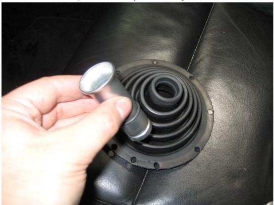
...and push the new Forge adaptor into the gaitor from underneath, exposing as many threads as possible.
