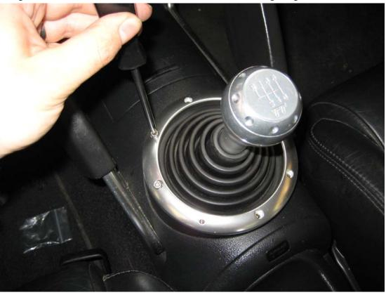
...then lift the ring away to expose the rubber underneath
