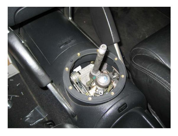
3. Push the old aluminium spacer out of the top of the rubber gaitor.....
