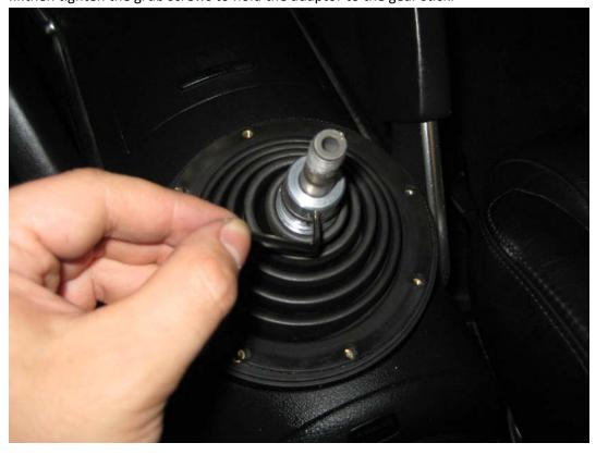
5. Replace the trim ring around the gaitor and screw the new knob down as far as it will go. The top of the gear stick should be just below the top of recess inside the top of the knob.
