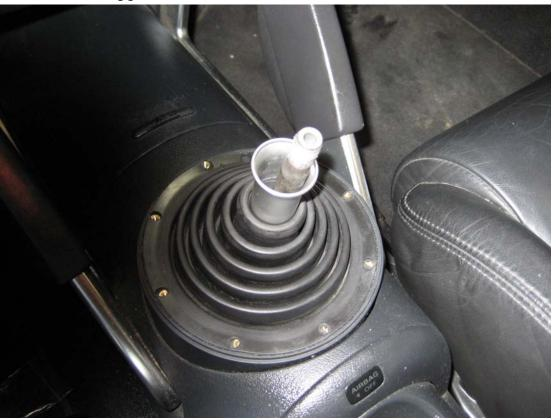
....and remove the rubber gaitor and aluminium spacer from the gear stick.
